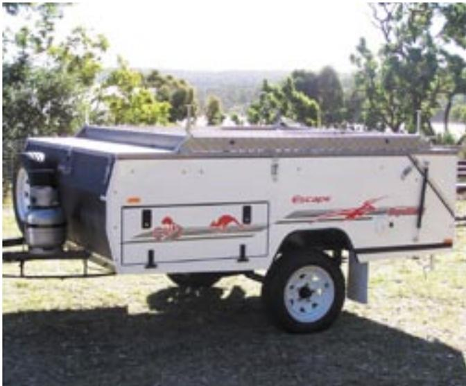
The Supamatic Escape has the same basic principle of a flip over camper and is designed for on road use. Cub has off road models and we will be reviewing them in upcoming issues. The Supamatic has a lightweight but strong construction that allows quite a large amount of internal space.
